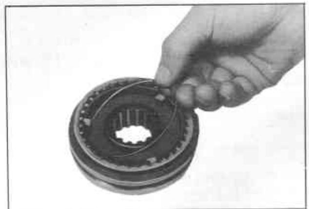
*Fig. TM-32 2nd and 3rd synchronizer*
