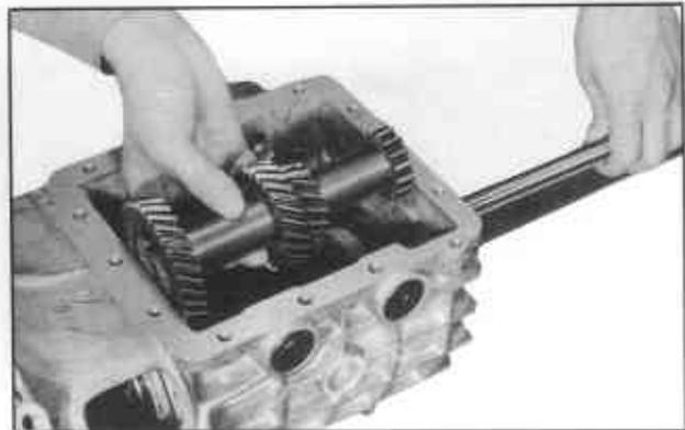
*Fig. TM-14 Counter gear removal*
