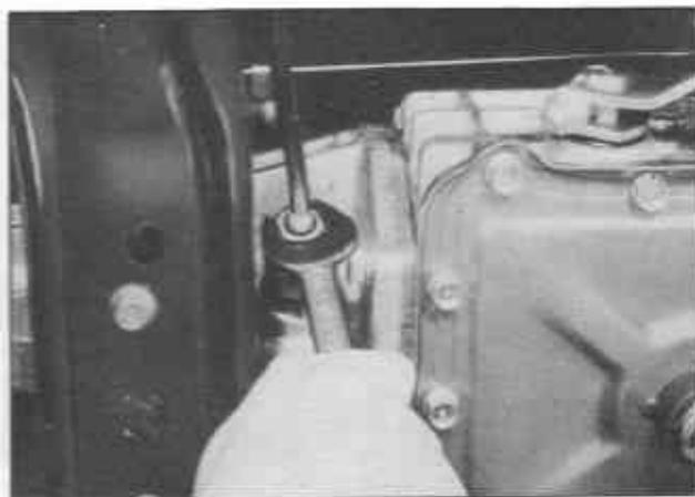
*Fig. TM-7 Disconnecting speedometer cable*
